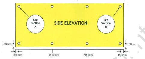
3. If this is not practicable, the ventilation holes can be fitted in both ends (as indicated below). All dimensions are taken from inside the steel storage container.
